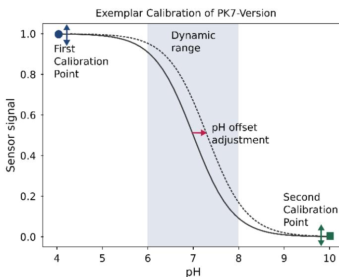
Do not use commercially available buffer solutions used for pH electrodes. These buffers (colored and uncolored) will affect the sensor performance irreversibly due to stabilizers in the solution. It is important to only use **PyroScience** buffer capsules or self-made buffers with known pH and ionic strength for calibration (with advice from **PyroScience**).
