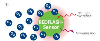
**Principle:** red light excited REDFLASH indicators show luminescence in the near infrared (NIR), which decreases with increasing oxygen (quenching effect).
