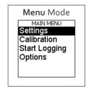
After exiting the menu mode with the BACK button, the device reverts to the Live Mode. For details on the menu mode refer to chapter 6.
