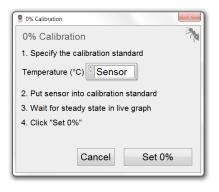
(1) Temperature Compensation. Select now the mode of temperature compensation used during o% calibration by clicking on Temperature (°C). For automatic temperature compensation with the PT100 temperature sensor connected to the *FireStingGO*2 device, select Sensor.
