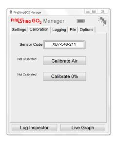
For highest precision it is recommended to calibrate both calibration points. However, if the expected measuring range is close to of the calibration points, then a 1-point calibration might be sufficient. For example if the expected measuring range in a liquid sample is 95-100% air sat., then a 1point calibration at saturated water is typically
