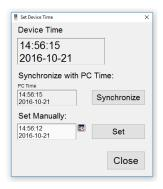
If it is incorrect, click on **Set Device Time**. This opens a window for adjusting the device time. Clicking on **Synchronize** will set it to the PC Time. Alternatively the time and date can be adjusted manually. For this, edit the time and date below "Set Manually", and click on **Set**.
