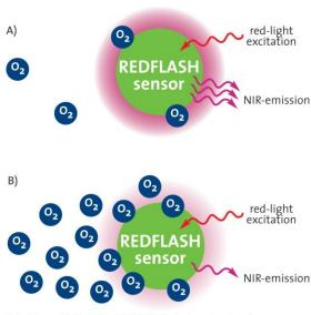
**Principle:** red light excited REDFLASH indicators show luminescence in the near infrared (NIR), which decreases with increasing oxygen (quenching effect).
