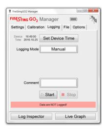
that the device is configured and calibrated with the *FireStingGO2 Manager*, then logging is started and the device is disconnected and deployed at the measurement location. Later when the measurements are completed, the device is again connected to the PC, and the logged data are downloaded and inspected. The following steps must be done for data logging:
