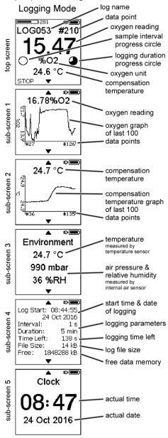
In sub-screen 2 the last 100 data points of the compensation temperature are displayed in a graph. The last logged compensation temperature is shown additionally as numerical value.
