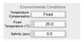
**IMPORTANT**: For measurements with a **Fixed** temperature, the temperature in the sample must be measured and kept constant during the entire measurement!
