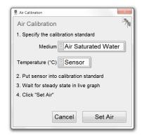
the gas phase, it is advised to choose **Ambient Air** and to continue with step (2A). If the measurements will be done in aqueous samples, it is advised to choose **Air Saturated Water** and to continue with step (2B).
