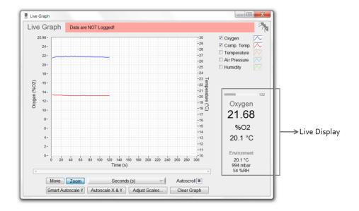
The Live Display shows numerical live readings of all sensors comprising oxygen, compensation temperature, temperature (if a temperature sensor is connected), and the readings of the internal
