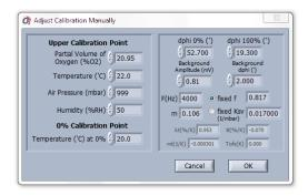
Here the Upper Calibration Point (default: Partial Volume of Oxygen 20.95% O2) can be defined, as well as the calibration conditions (Temperature, Air Pressure, Humidity) as described for the Custom Calibration (see chapter 7.1.6). The Temperature (°C) needs also to be determined and entered for the o% Calibration Point.
