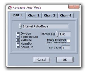
Three options can be selected. The first option **Disable Auto-Mode** disables any measurement in the auto-mode for the respective channel (but it does not disable the auto-mode in general!). For the second option **Interval Auto-Mode**, the sample **Interval (s)** can be adjusted for each channel independently. If the last option **Triggered Auto-Mode** is chosen, the measurement of the
