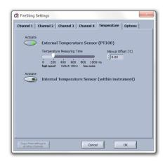
Both temperature sensors can be activated independently even if **Fixed Temperature** or **Optical Temperature Sensor** was selected for temperature compensation of all connected oxygen sensors (in this case the oxygen measurements are not affected by these temperature sensor measurements). The measured temperature is then displayed in the **Overview** panel (see chapter 6.3) of the main window and saved into the data file (see chapter 6.4).
