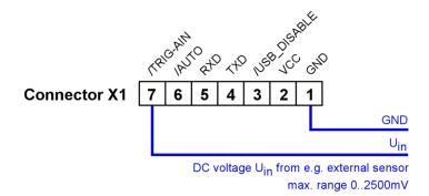
For reading in voltage signals between o and 2.5 VDC of e.g. an external sensor, simply connect the voltage to pin 1 and pin 7. Ensure a correct polarity. And ensure that the voltage does not exceed 2.5 VDC. Voltages above 3.3 VDC might damage the device.
