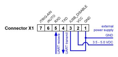
This configuration is used if the *FireStingO2* should be controlled completely via the UART interface by external custom electronic equipment (OEM applications). Note the additional connection between pin 1 and 3 powering down the internal USB interface of the *FireStingO2*. Otherwise unintended data communication via a potentially still connected PC might disrupt the UART communication. More information is available on request.
