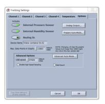
The activation of the **Analog In** button allows to read in a voltage signal at the extension port, e.g. from third-party sensors. The
