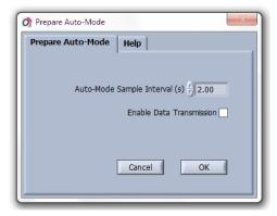
Here the **Auto-Mode Sample Interval (s)** can be adjusted, defining the time interval between consecutive measurements in the automode. As an advanced feature, the option **Enable Data Transmission** activates digital data transmission via the UART interface of the extension port (details on request).
