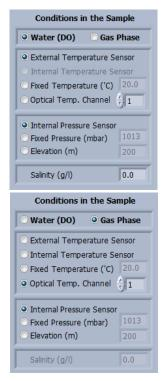
For **Gas** measurements, temperature could be measured in principal also by the **Internal Temperature Sensor** of the *FireStingO2*, but this is **NOT** recommended!
