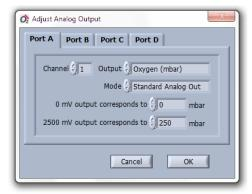
The settings of the 4 analog outputs can be adjusted in the respective tabs designated as **Port A-D**.
