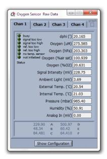
The panels of each oxygen channel (Chan 1-4) show the phase shift as "delta phi" (dphi, in °). dphi is the actual measured raw value which is used for the internal calculation of the oxygen concentration Oxygen (µM), Oxygen partial pressure (hPa), Oxygen in % air saturation (% air sat) and Oxygen (% O2) (see also chapter 12.4).
