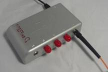
First, remove the black caps from the plug of the sensor / fiber. Then remove the red caps from the sensor ports at the *FireStingO2* (the red caps should be put on again if the *FireStingO2* is not in use anymore to protect the optics). Insert the male fiber plug of the sensor cable into the ST-port (female fiber connector) of the *FireStingO2* and turn the bayonet coupling gently clockwise until the plug is locked firmly.
