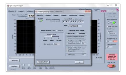
Activate each connected sensor in the respective channel tab of the **Settings** window, corresponding to the channel number at the *FireStingO2* meter (see chapter 3). Enter the **Sensor Code** and all relevant parameters (**Units, Measuring Mode, Conditions in the Sample**) into **each** channel tab before calibration and measurements, as described in detail in chapter 6.1.
