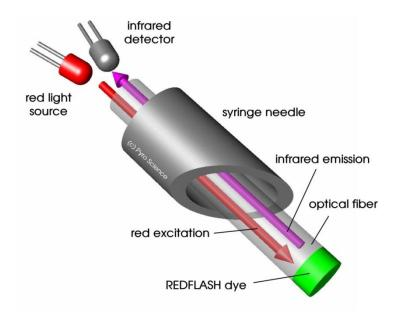
The measuring principle is based on a sinusoidally modulated red excitation light. This results in a phase-shifted sinusoidally modulated emission in the NIR. The *FireStingO2* measures this phase shift (termed "dphi" in the software). The phase shift is then converted into oxygen units based on the Stern-Vollmer-Theory.
