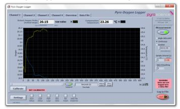
The four panels **Channel 1-4** correspond to the fiber-optic sensors connected to the ports **1-4** at the *FireStingO2* (see chapter 3). For the 1- or 2-channel version of the *FireStingO2*, only the respective panels will be visible.
