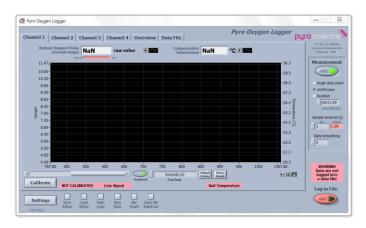
If a sensor is not yet calibrated, the warning **Not Calibrated** is shown on the right-hand side of the **Calibrate** button and the data are shown in units of "raw value", reflecting the measured oxygen levels only qualitatively. In order to switch to **quantitative** oxygen units, a sensor calibration has to be performed by clicking on **Calibrate**. The calibration procedure is explained in detail in chapter 7.
